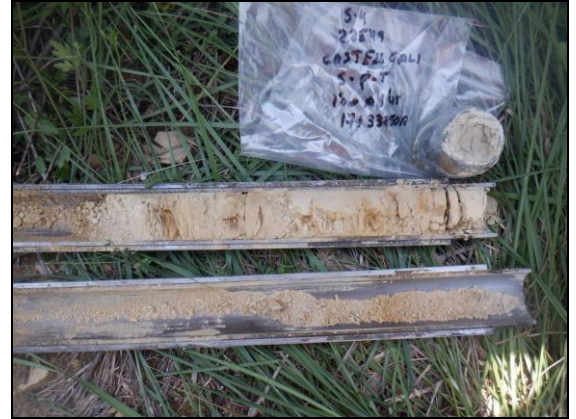
Foto 8: Sondeig S-4, SPT a 1,0 metre.
