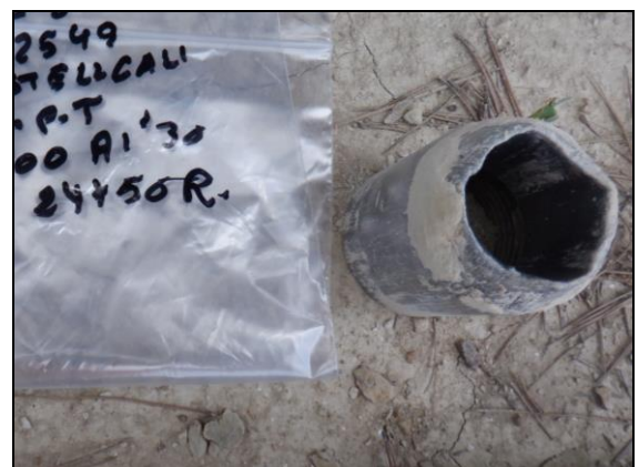
Foto 18: Sondeig S-9, SPT a 1,0 metre.
