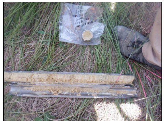
Foto 10: Sondeig S-5, SPT a 1,0 metre.
