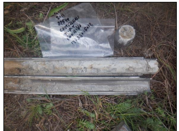
Foto 22: Sondeig S-11, SPT a 1,0 metre.
