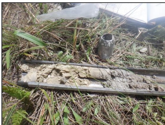
Foto 33: Sondeig S-15, SPT a 1,0 metre.
