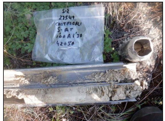
Foto 4: Sondeig S-2, SPT a 1,0 metre.
