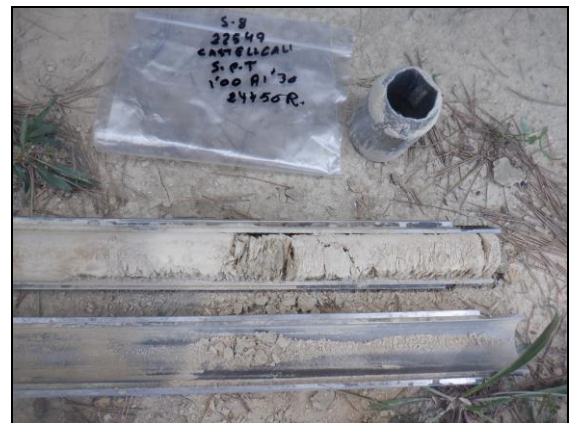
Foto 16: Sondeig S-85, SPT a 1,0 metre.
