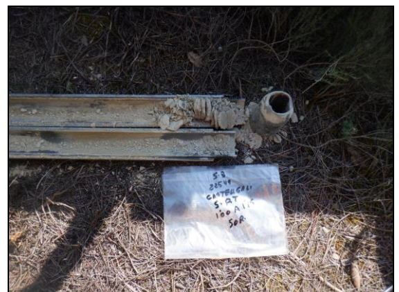
Foto 6: Sondeig S-3, SPT a 1,0 metre.
