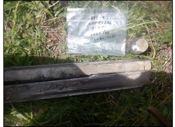
Foto 26: Sondeig S-12, SPT a 1,0 metre.
