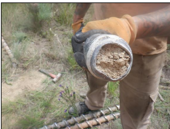
Foto 29: Sondeig S-13, SPT a 1,0 metre.
