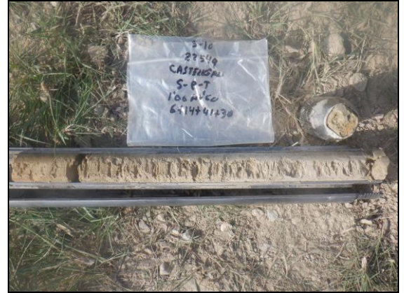
Foto 20: Sondeig S-10, SPT a 1,0 metre.
